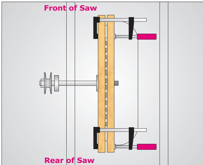
One method you may want to try is shown in the drawing to the left. Make 2 pieces of pine about 3” wide, and longer than the throat opening on the saw. The blade should be square to the saw top. Install an old blade on the saw, and tighten to normal pressure. Raise the blade to the height of the pieces, and firmly clamp the saw blade between the wood strips..
