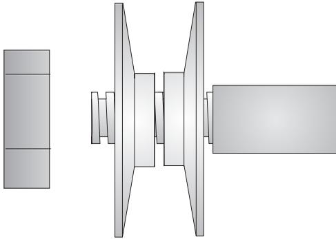
Where most contractor saws use “slip-on” pulleys, Delta contractors and the DeWALT 746 hybrid take a different approach, as the arbor shaft is threaded on both ends. The arbor shaft is a larger diameter than most contractor saw arbors, and is reduced in diameter to accept a 5/8” bore blade and pulley. The face of the shaft on the pulley end where the reduction in size takes place serves as a “stop” where the inside face of the pulley will make contact.
