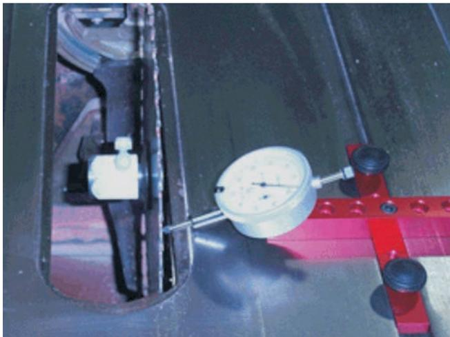
**A-LINE-IT Set-up on a right-tilt saw**
