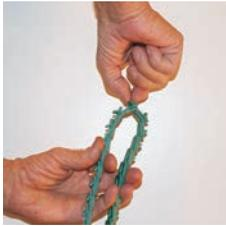
With the tabs out, and the belt upside down, twist one tab 90°, parallel
