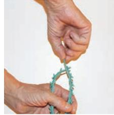
Flex the belt further and insert the 2nd tab through the end link by
