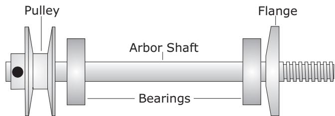
As the alignment procedure is performed, we will show how to do the most accurate procedure to make the test. The technique allows you to determine if the arbor shaft on the saw is square to the miter slots on the saw, which is mandatory if you want the blade to be perfectly parallel to the slots.
