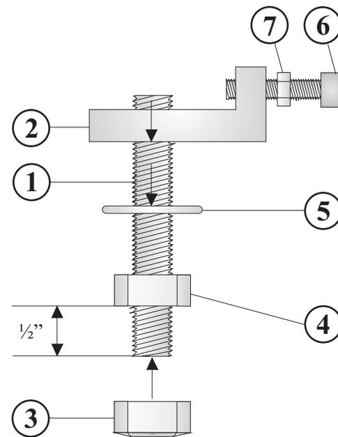
When I installed the “prototype” PALS on my contractor saws, I wanted to make sure that I did everything I could to make the procedure as easy as possible. Since the movement of the original bolts contributed to the trunnion moving, I wanted to insure that the studs couldn’t turn as I tightened the nuts on the PALS.
