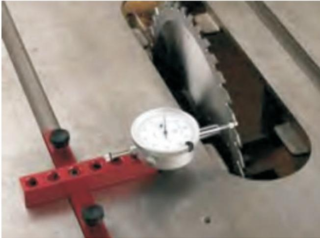
**A-LINE-IT Set-up on a left-tilt saw**
