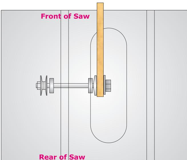
If the technique above doesn’t work, the method shown in the drawing to the left should. Bore a 5/8” hole through one piece of pine. Remove the saw blade, and moisten the area around the hole in the pine with water. Place the piece on the arbor, and install the blade washer and nut. Tighten the nut as you normally would for using a blade. Rotate the piece to make contact with front of the throat opening.
