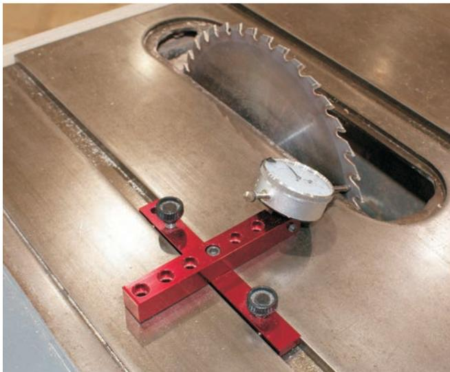
**Step 1.** Configure the A-Line-It as shown in the photo to the left, in the miter slot of your choice. Note that the tip of the indicator is pointing downward. This is done to increase the distance point-to-point as we rotate the blade front-to-rear. This makes the error in our alignment more obvious.
