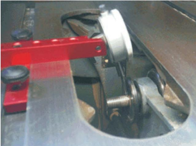
For your saw to operate properly, the “business end” of the saw must be in good mechanical condition. This means that the arbor shaft should be straight, and the arbor shaft bearings must be in good condition.
