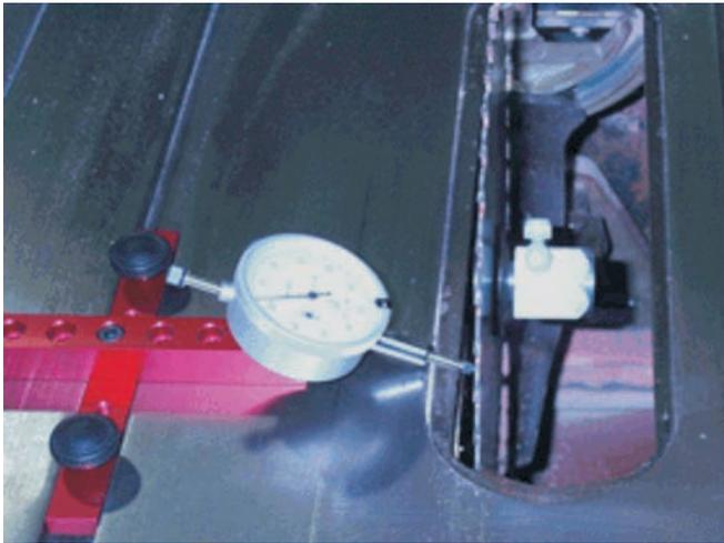
**A-LINE-IT Set-up on a left-tilt saw**
