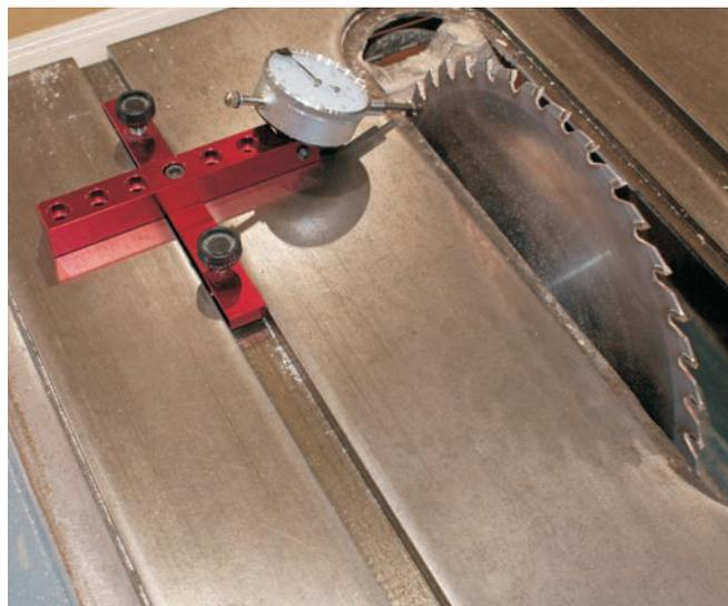
**Step 3.** Slide the indicator toward the rear of the saw as you rotate the blade toward the rear of the saw, as shown in the photo to the left. Align the tip of the indicator on the dot on the blade, and note the reading shown.
