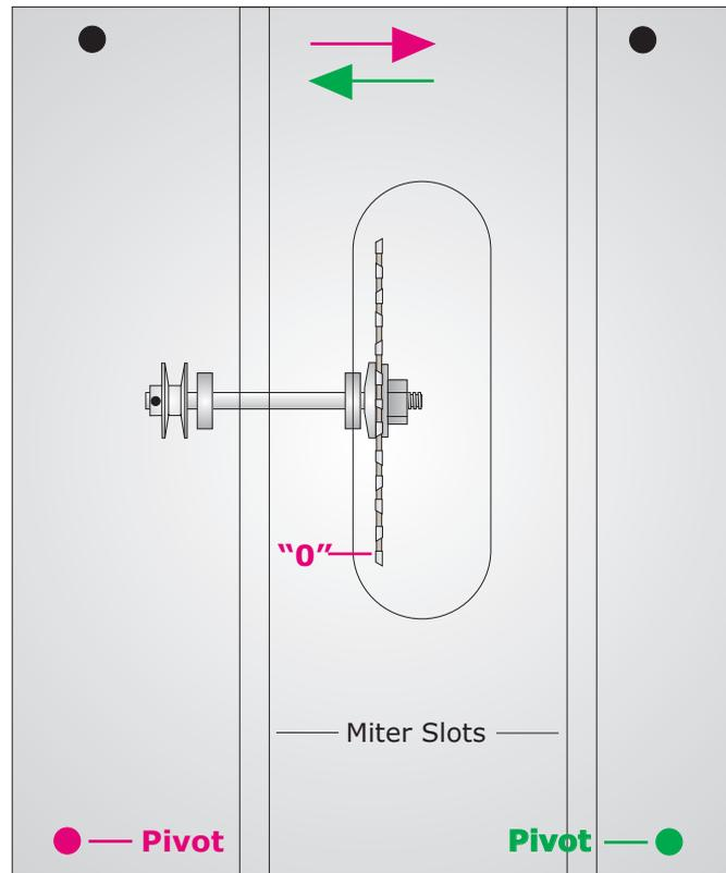
On these saws, the rear bolt is the "pivot point".
