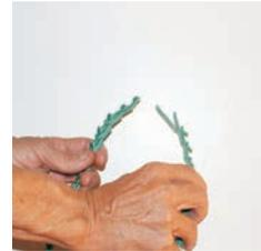
Pull the belt end with the tab through two links to separate the
