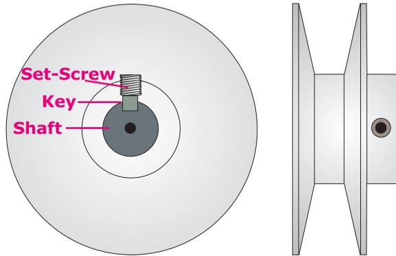
Replacing the standard pulleys and belt with machined steel pulleys and a “link belt” will make quite a difference in the performance of contractor style saws, on which the motor weight is used to determine the tension on the belt.
