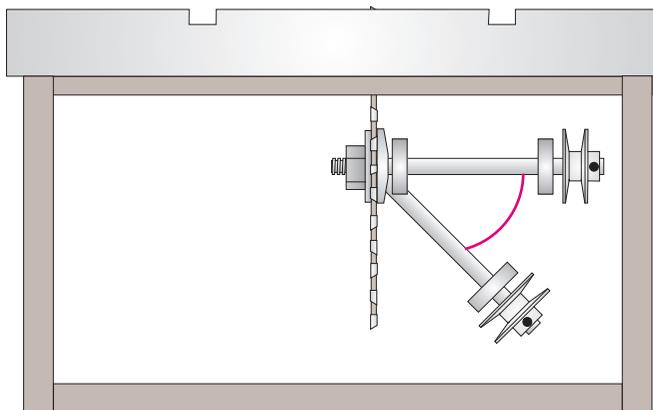
There is normally very little clearance between the pulley and the cabinet of the saw when the blade is square to the top of the saw.
